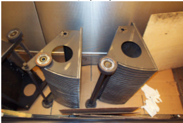
Pictured: Broken flange brackets required custom fabrication to repair/replace.
